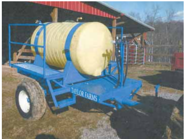
Alfred Taylor's pull-type boomless sprayer is equipped with a 300-gal. spray tank and a rear-mount broadcast nozzle that covers 60 ft. in a pass.
